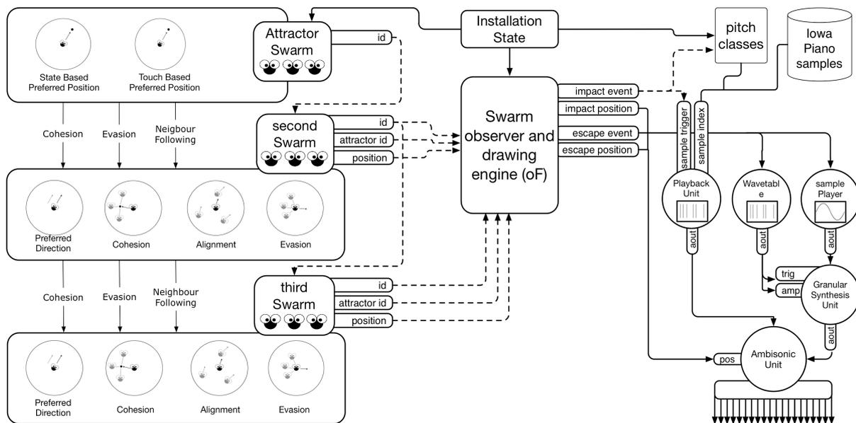
**Figure 1.** Schematics of the swarm music piece “Impacts”. The hierarchy of the swarm simulations is depicted on the left side. The intermediate mapping stage performs the analysis of swarm behavior and generates the control events and data for the musical engine, which is shown on the right.
