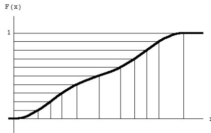
Figure 8. Uniformly distributed random values in  $F(x)$  correspond to random numbers  $x$  with the density  $f(x)$ .
